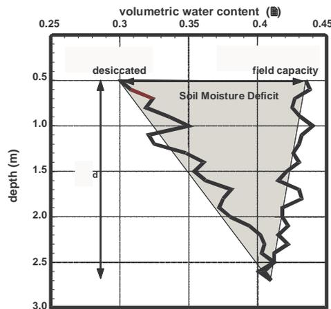
Figure 3: Illustration of Soil Moisture Deficit in the ground for a desiccated profile and a profile at field capacity.
