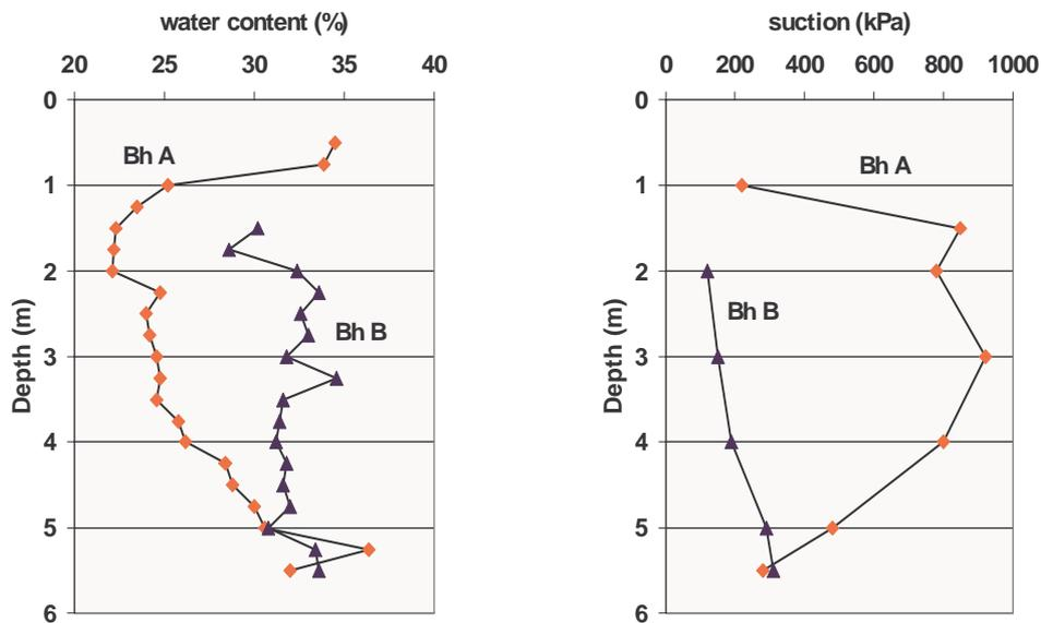
Figure 2: Typical profiles of water content and suction in a desiccated location (A) and a normal location (B), after BRE (1996.)
