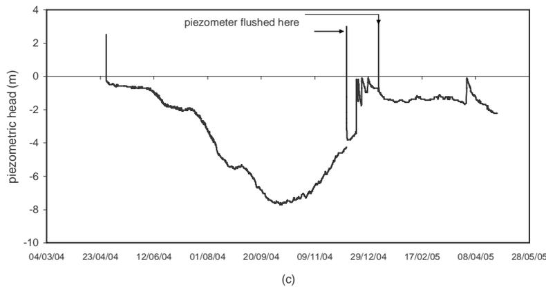
Figure 6: GeO Piezo Suction Measurements at Chainage 600 on Lockwood Reservoir (a) depth 1.04m between Design TWL and Target TWL, (b) depth 1.64m between Target TWL and Restricted TWL, and (c) depth 2.48m below Restricted TWL.
