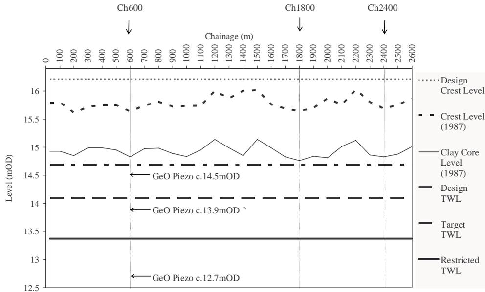
Figure 5: Long Section for Lockwood Reservoir, showing TWL, Clay Core Level and locations of the GeO Piezo's.
