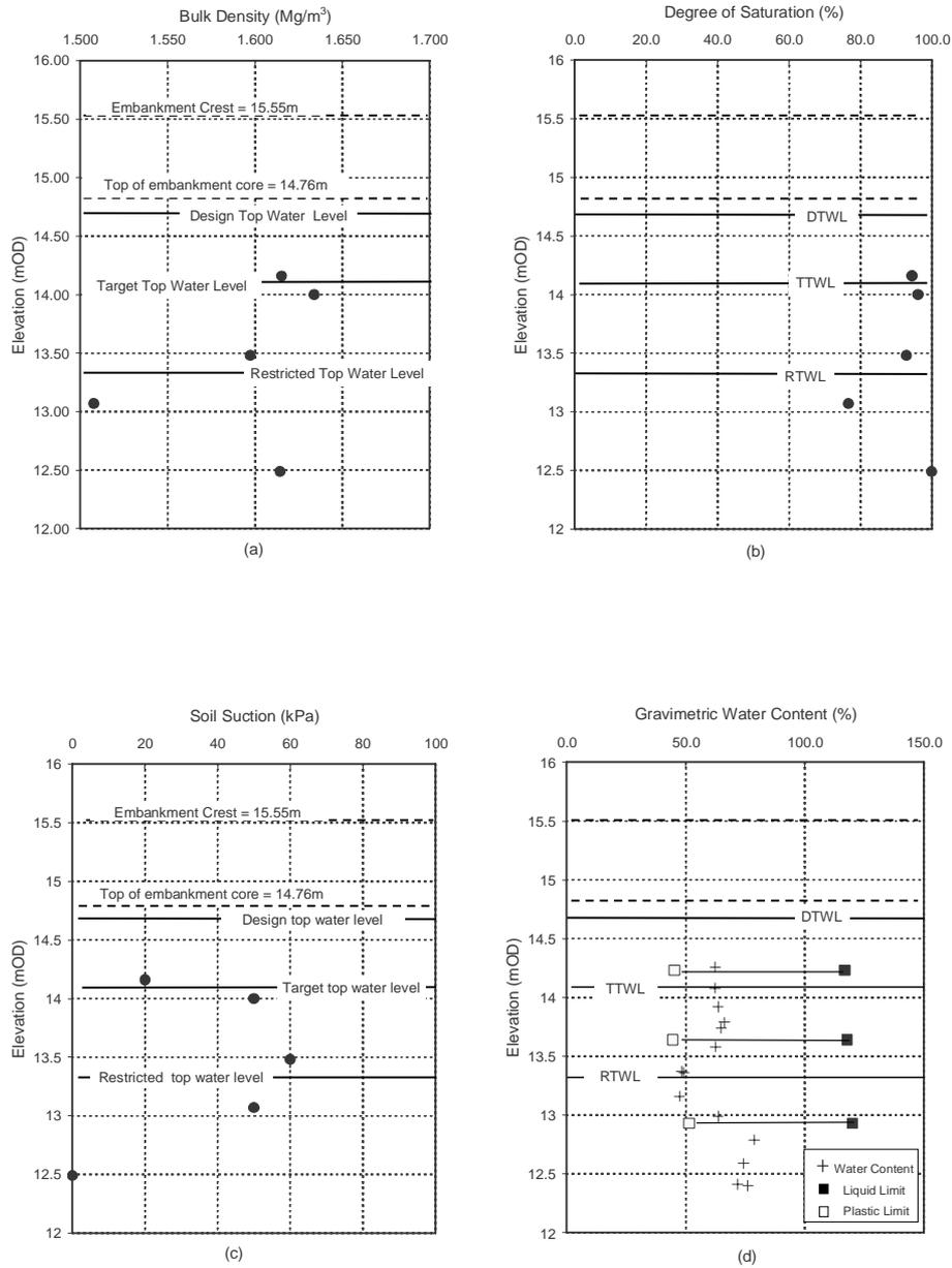
Figure 4: Laboratory Test Results on samples of clay core from Chainage 600 on Lockwood Reservoir (a) Bulk Density, (b) Degree of Saturation, (c) Soil Suction and (d) Gravimetric Water Content.
